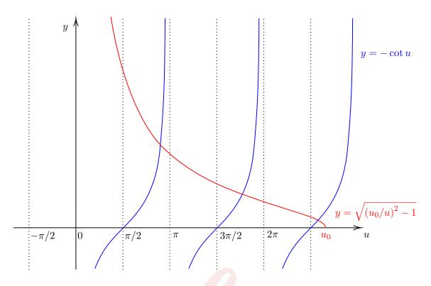
Again, we find only a finite number of intersections. The number of odd bound state is bigger for larger  $u_0$ , i.e., for wider and deeper well. However, for  $u_0$  sufficiently small, say  $u_0 < \pi/2$ , there will be no odd bound state.
